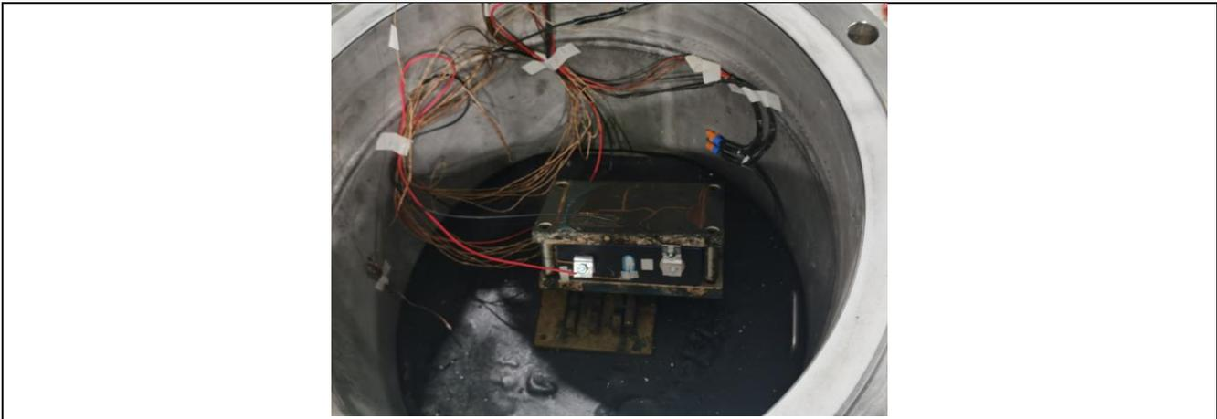
Figure 21: Sample 5 instrumented and inside gas test chamber
